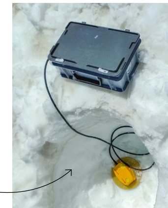
Traditional measuring method with a geophone and data logger (inside box)
